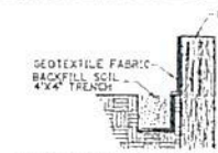
SECTION THRU TRENCH SHOWING GEOTEXTILE FABRIC
